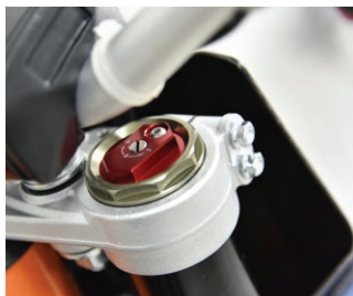
Adjustable front suspension & rear shock (chrome plated core)
